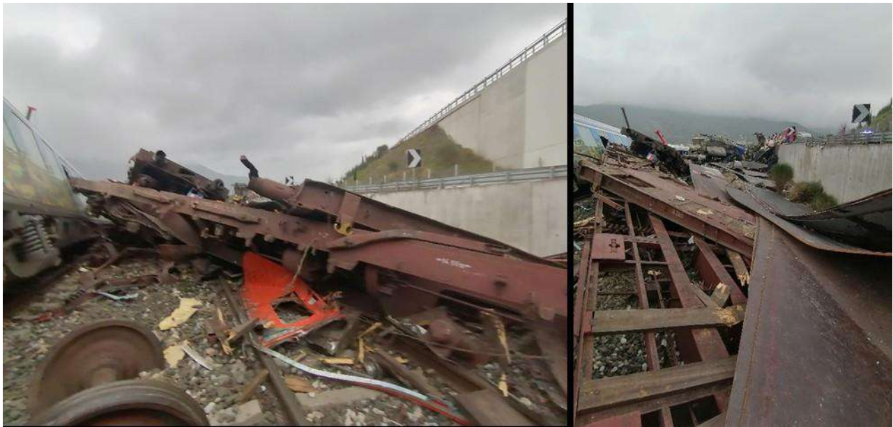
Figure 82. Platforms as found on the accident site.
