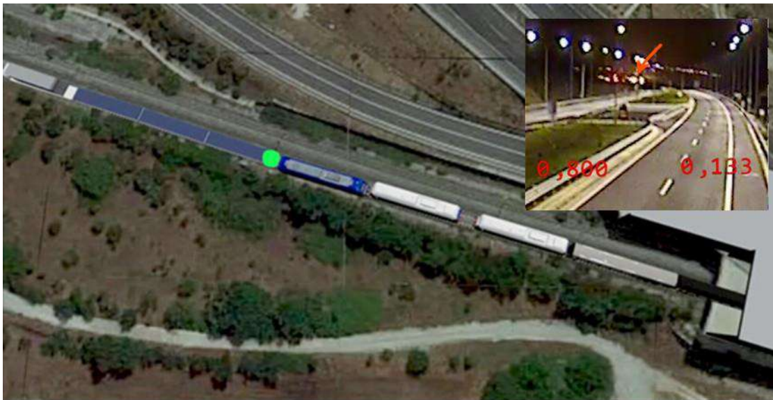
Figure 58. Estimated point of initial ignition.
